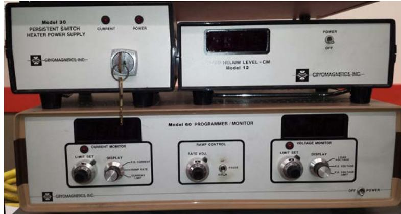
**Figure 7:** The Model 30 Persistent Switch, Model 12 LHe Level indicator and Model 60 Programmer/Monitor power supply controller
