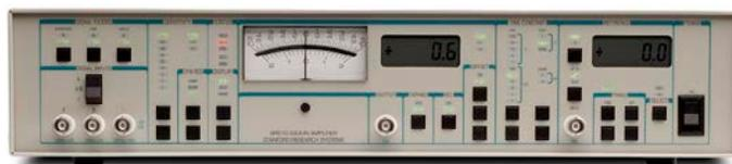
**Figure 6:** The SR510 lock-in amplifier
