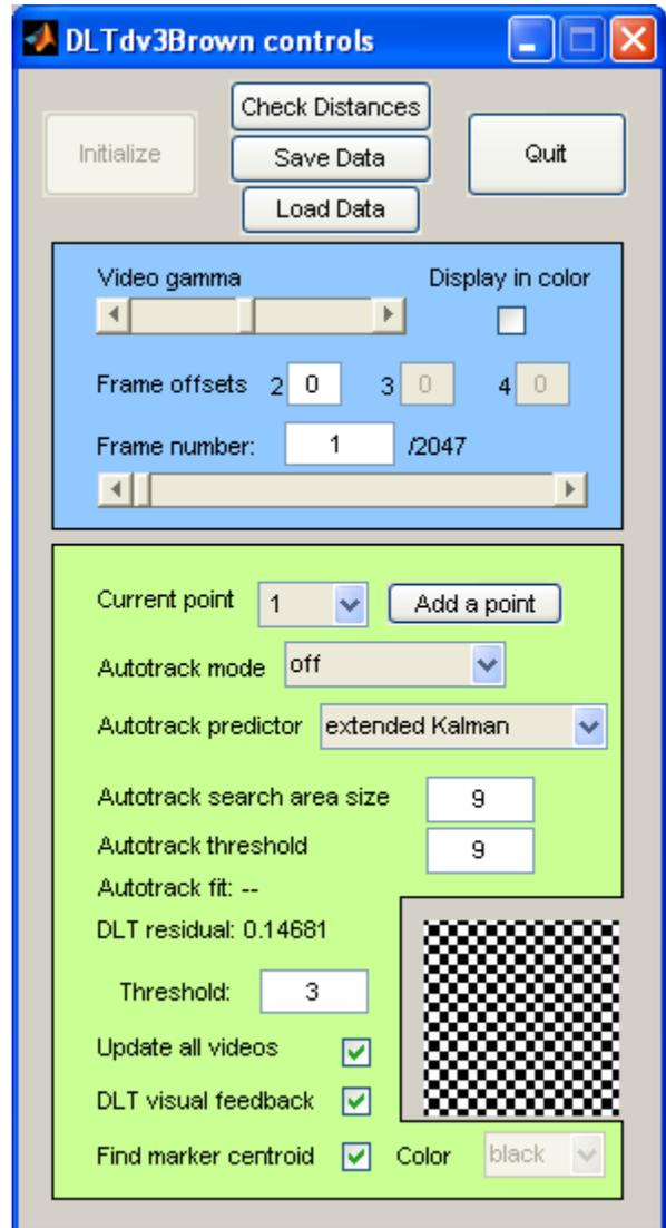
**Autotrack fit:** During autotracking, as long as this value is greater than the autotrack threshold, the computer will continue autotracking
